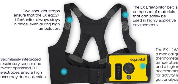
The EX LifeMonitor includes a medical grade infrared thermometer that measures temperature every 15 secs and a high resolution tri-axis accelerometer providing data for activity monitoring and gait analysis.
