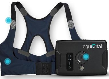
The LifeMonitor includes a medical grade infrared thermometer that measures temperature every 15 secs and a high resolution tri-axis accelerometer providing data for activity monitoring and gait analysis.
